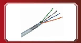
Enhanced performance cable for transmission of high speed data, digital and analogue voice and video (RGB) signals on LANs. Supports Gigabit Ethernet (1000 baseT) standard. Operates at bandwidth of 100MHz. Tinned Copper Screening gives Protection against EMI and avoid signal loss. Better Mechanical Properties of Cable. This cable well exceeds the requirements of TIA/EIA-568.C.2
