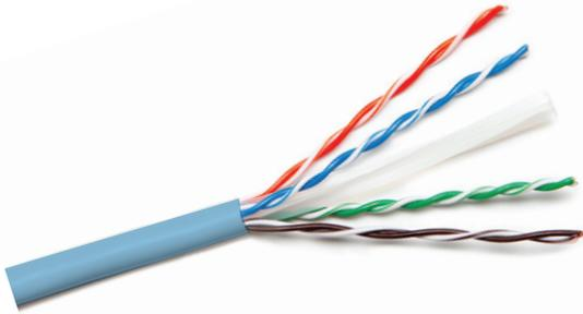
Enhanced performance cable for transmission of high speed data, digital and analogue voice and video (RGB) signals on LANs. Supports Gigabit Ethernet (1000 baseT) standard. Operates at bandwidth of 250MHz. This cable well exceeds the requirements of ANSI/TIA-568-C.2 and ISO/IEC 11801.
