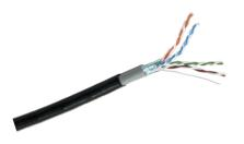
Enhanced performance cable for transmission of high speed data, digital and analogue voice and video (RGB) signals on LANs. Supports Gigabit Ethernet (1000 baseT) standard. Operates at bandwidth of 250MHz. The shield acts as a Faraday cage to reduce electrical noise from affecting the signals, and to reduce electromagnetic radiation that may interfere with other devices. This cable well exceeds the requirements of TIA/EIA-568-C.2 and ISO/IEC 11801.
