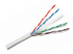
Enhanced performance cable for transmission of high speed data, digital and analogue voice and video (RGB) signals on LANs. Supports Gigabit Ethernet (1000 baseT) standard. Operates at bandwidth of 250MHz. This cable well exceeds the requirements of TIA/EIA-568-C.2 and ISO/IEC 11801
