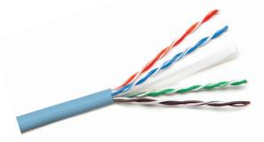
Enhanced performance cable for transmission of high speed data, digital and analogue voice and video (RGB) signals on LANs. Supports Gigabit Ethernet (1000 baseT) standard. Operates at bandwidth of 250MHz.
