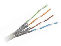
Enhanced performance cable for transmission of high speed data, digital and analogue voice and video (RGB) signals on LANs. It supports Gigabit Ethernet (10GbaseT) standard and operates at bandwidth of 500MHz. This cable well exceeds the requirements of ANSI/TIA-568-C.2. The shield acts as a Faraday cage to reduce electrical noise from affecting the signals, and to reduce electromagnetic radiation that may interfere with other devices.
