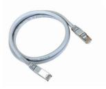
D-Link Cat6 STP patch cords are high quality four pair shielded twisted stranded cable terminated with RJ45 modular plugs at both the ends. It is TIA/EIA 568C.2 standard. The shielded cables helps to complete a proper ground connection and allows longer runs with less effect of Electromagnetic Interference (EMI) and Radio Frequency Interference (RFI). These patch cords are appropriate for high speed data transmission.
