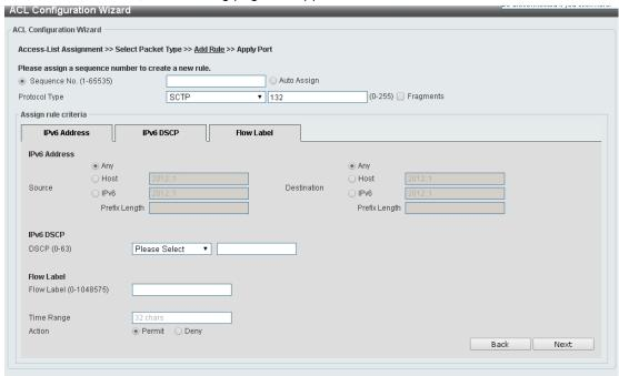
Figure 4.143 – ACL > ACL Configuration Wizard – Create IPv6 ACL-SCTP
