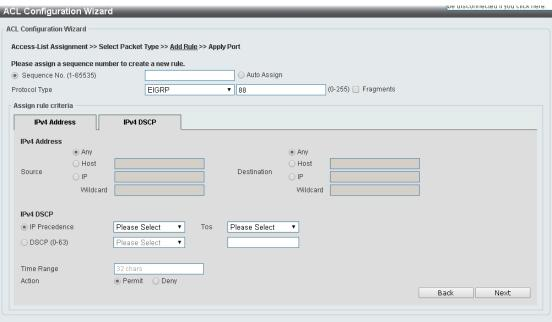
Figure 4.126 - ACL > ACL Configuration Wizard - Create IPv4 ACL-EIGRP
