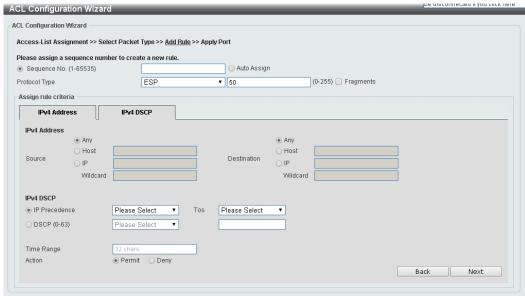
Figure 4.127 – ACL > ACL Configuration Wizard – Create IPv4 ACL-ESP
