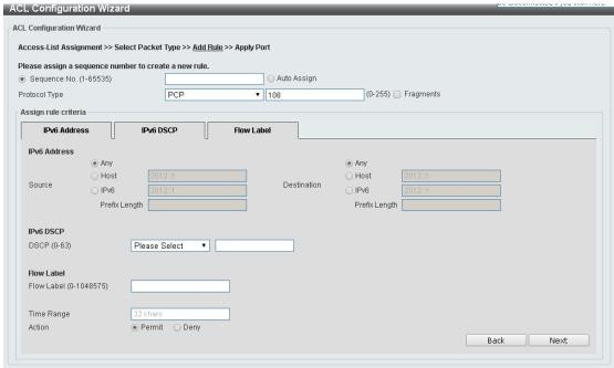
Figure 4.142 – ACL > ACL Configuration Wizard – Create IPv6 ACL-PCP
