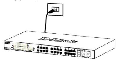
Figure 2.4 –Plugging the switch into an outlet
