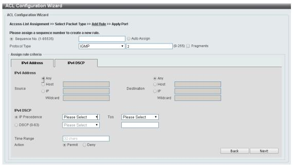
Figure 4.129 - ACL > ACL Configuration Wizard - Create IPv4 ACL-IGMP
