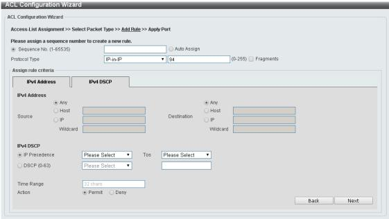
Figure 4.133 - ACL > ACL Configuration Wizard - Create IPv4 ACL-IP in IP
