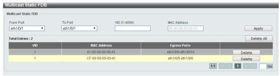
Figure 4.58 - L2 Features > FDB > Static FDB > Multicast Static FDB
