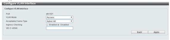
Figure 4.66 - L2 Features > VLAN Interface - VLAN Detail
