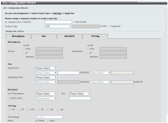
Figure 4.123 - ACL > ACL Configuration Wizard - Create IPv4 ACL-TCP
