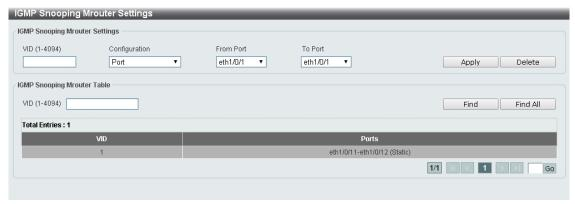
Figure 4.78 - L2 Features > L2 Multicast Control > IGMP Snooping > IGMP Snooping Mrouter Settings
