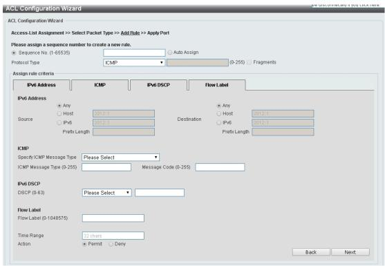
Figure 4.139- ACL > ACL Configuration Wizard - Create IPv6 ACL-ICMP
