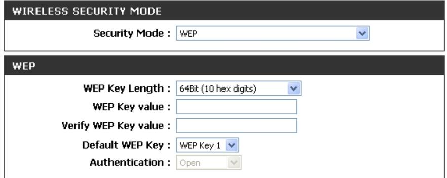
The screenshot displays the 'WIRELESS SECURITY MODE' configuration page. The 'Security Mode' is set to 'WEP'. Below this, the 'WEP' section is expanded, showing the following settings: 'WEP Key Length' is set to '64Bit (10 hex digits)', 'WEP Key value' and 'Verify WEP Key value' are empty text input fields, 'Default WEP Key' is set to 'WEP Key 1', and 'Authentication' is set to 'Open'.
