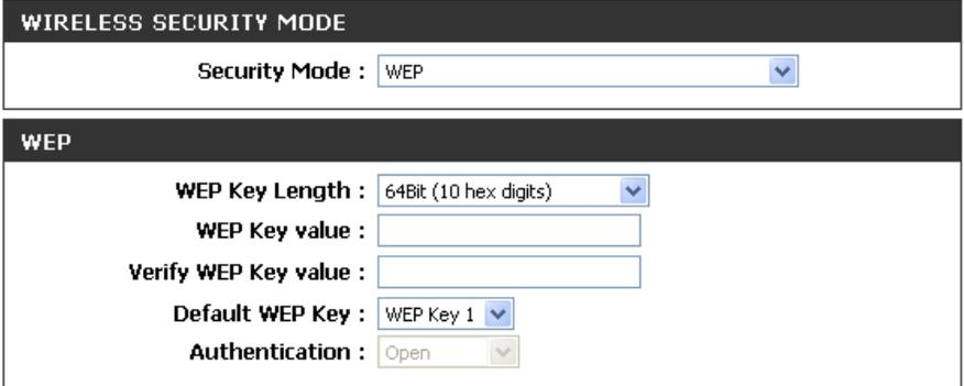
The screenshot shows the configuration interface for WEP. It is divided into two sections: 'WIRELESS SECURITY MODE' and 'WEP'. In the 'WIRELESS SECURITY MODE' section, 'Security Mode' is set to 'WEP'. In the 'WEP' section, 'WEP Key Length' is set to '64Bit (10 hex digits)'. There are two empty text input fields for 'WEP Key value' and 'Verify WEP Key value'. 'Default WEP Key' is set to 'WEP Key 1' and 'Authentication' is set to 'Open'.
