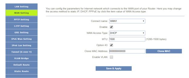
There are four wan connection can be use, each wan connection can be configured as difference mode, such as DHCP router mode, PPPoE router mode, Static router mode, and each wan connection can be configured to have VLAN tag, this will more helpful for user to meet different environment usage.
