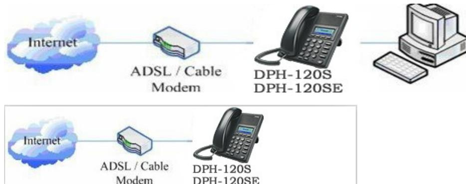
Shared network connection—Use this method if you have a single Ethernet port in your workspace with your desktop computer already connected to it. First, disconnect the Ethernet cable from the computer and attach it to the WAN port on the back of your phone. Next, use the Ethernet cable in the package to connect LAN port on the back of your phone to your desktop computer. Your IP Phone now shares a network connection with your computer. The following figure is for your reference.
