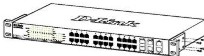
Figure 2.2 – Attach the mounting brackets to the Switch
